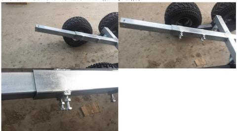
11.) Frame rail should extend approximately 40" passed main frame, tighten all 4 bolts and then all 4 nuts.
