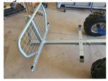
16.) Install outriggers and retaining handles.
