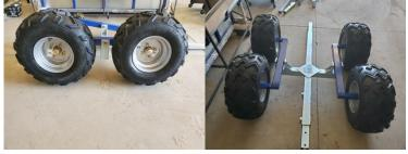
9.) Flip frame section over so that the frame is higher than the walking beams and slide frame rail in.
