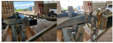
33.) Tighten bolt holding chains to boom.
