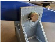
7.) Grease both pins liberally using a grease gun.
