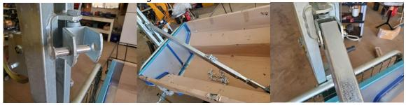
31.) Remove chain locking pins from swivel plate.
