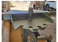
28.) Remove bolt holding winch cable roller, run winch cable through and re-install roller, tighten nut & bolt.
