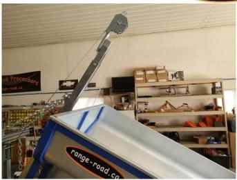
Loosen 4 main frame bolts and pull inner tube forward or backward to make frame length shorter or longer.
