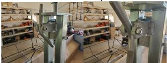
27.) Install Swivel plate, tighten the nut so that it locks but plate must move freely, install spring around lock lever and through the hole in the plate.
