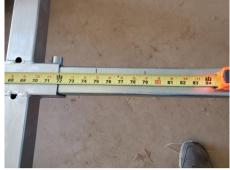
15.) Slide safety cage section onto front of frame, it should sit about 80  $\frac{1}{2}$ " from rear hinges, install 2 large bolts and nuts.
