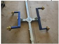
8.) Install all 4 tires, R oin one side L on the other and tighten wheel nuts to 40ft/lbs.
