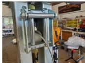
30.) Mount crane arm to frame hinge mount.
